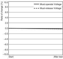
Characteristics were measured after applying vibration at a frequency of 5 to 200 to 5Hz, acceleration of 44.1 m/s² to the test piece (not energized) for 2 hours each in 3 directions
