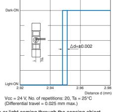
Note: The data applies to dark status. Operation may be affected by external light interference or light coming through the sensing object.
