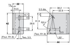
**Photoelectric Sensor** Accessory are installed (Example of E3AS-L200 ()
