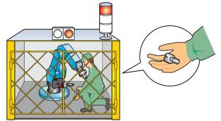
• Models with Rear Release Buttons A rear release button allows the door to be unlocked from inside a hazardous area in an emergency.
