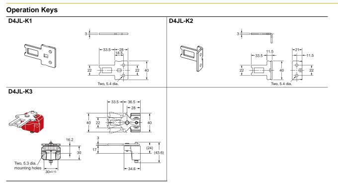
Note: Unless otherwise specified, a tolerance of ±0.8 mm applies to all Switch dimensions and a tolerance of ±0.4 mm applies to Operation Key dimensions.
