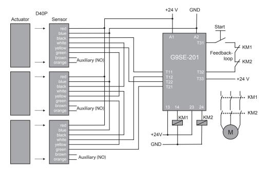
NOTE: For automatic reset connect the feedback loop between T31 and T33. Connect T32 to +24 VDC.
