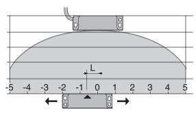
5 mm misalignment tolerance after setting
