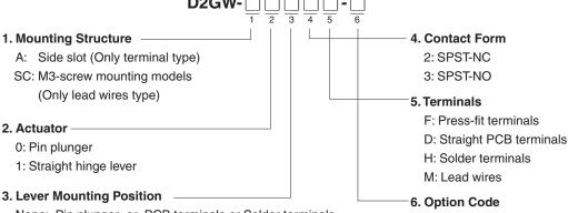
None: Pin plunger or PCB terminals or Solder terminals
