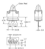
Insertion side unit mounting dimensions (for reference only)
