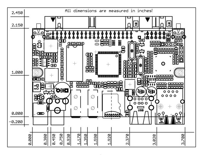
The three highest elements on the board in order from the tallest to the shortest are: inductor L2; USB host connector; Ethernet/LAN connector.
