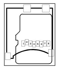
Notice that the pad numeration is written at the bottom of STM32-H407 under the microSD card connector.
