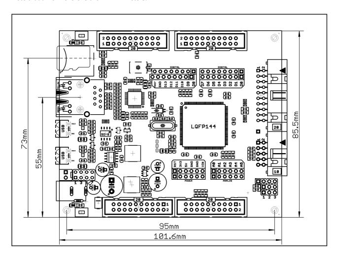
The three highest elements on the board in order from the tallest to the shortest are: capacitor C50 – 17.2mm (0.677") over the pcb; LAN connector – 13.6mm (0.535"); capacitors C42 and C48 – 11.5mm (0.453").
