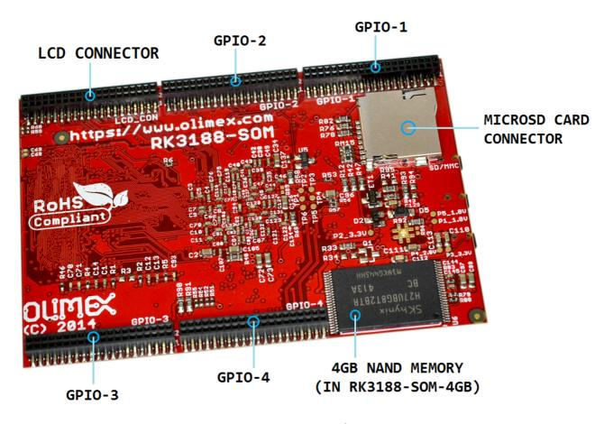
GPIO-1, GPIO-2, GPIO-3, GPIO-4, and LCD\_CON are female connectors with 0.01" step. They are used to attach RK3188-SOM to RK3188-SOM-EVB (or to your custom shield of peripherals).
