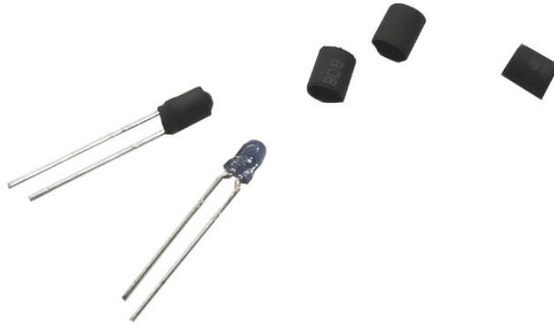
In the kit there are two rubber pads which can be used as vehicle tyres on each motors. We suggest to cut and use the smaller rubber pads as tyres, using the bigger pads will make robot faster but also not very stable.
