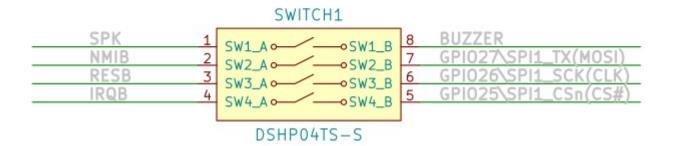
By default Neo6502 is shipped with all sections connected on the switch i.e. buzzer is enabled and all signals are wired to RP2040. This means you can't use SPI on UEXT connector if you do not disconnect these signals.
