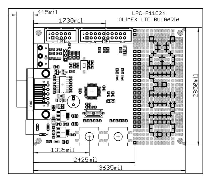
The three highest elements on the board in order from the tallest to the shortest are: RS232 connector – 480mil; capacitor C12 – 460mil; Power jack – 420mil.
