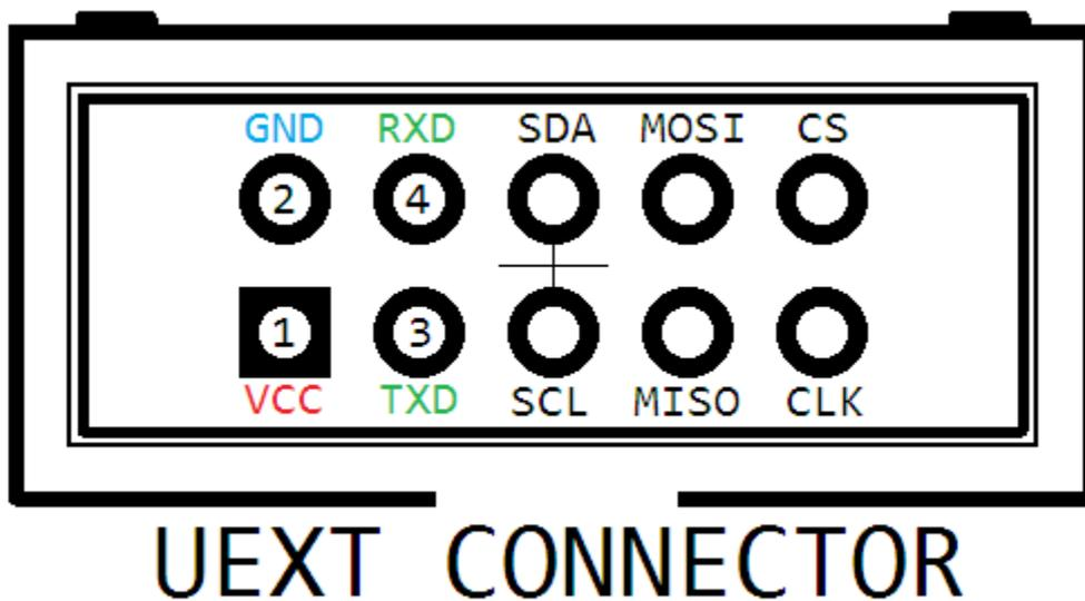
For connecting the USB<->serial cable we are interested only in pins #2, #3 and #4.
