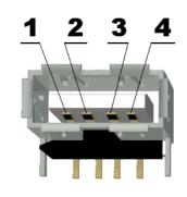
**USBMO** and **USBPO** form the differential input/output of the USB host 0. **USBM1** and **USBP1** form the differential input/output of the USB host 1.
