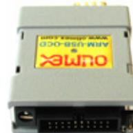
the power supply jumpers are on right side of the 2x10 pin JTAG connector.
