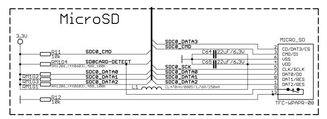
SD/MMC slot is a microSD card slot connector, located on the top of the board.
