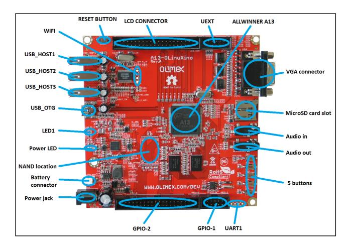
The picture above shows the initial revision of A13-OLinuXino. Note that the version of the board pictured does not have additional NAND memory nor WIFI module.
