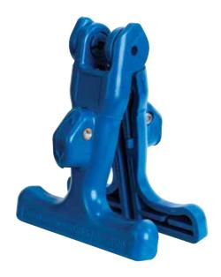
The FOD-2000 puts a slit on both sides of the jacket allowing easy access to the fiber or strength member. The ease of use makes this tool truly unique! To use just position the tool around the cable, pull and slit. A simple twist of the cable allows the jacket and strength members to separate from the buffer tube leaving the fiber undamaged.
