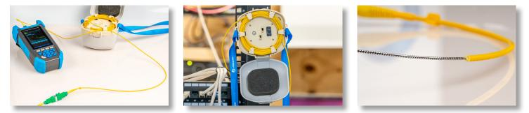
Designed with unique compact housings and 20-1000 meters of fiber, these launch cables are perfect for eliminating dead zones in reflectometric tests using an OTDR. These launch cable also features the following:
