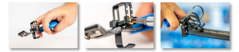
Designed to shave thick jacketed cable, such as Corning's armored and non-armored RocketRibbon<sup>®</sup> cable, this tool is perfect for making access windows on cables 0.47" to 0.87" (12 - 22 mm) in diameter. This tool also features the following:
