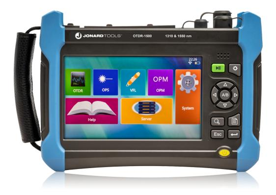
Jonard Tools' Professional Multi-Function OTDR is the perfect all-in-one handheld device for evaluating FTTx and access network construction and maintenance, identifying fiber breakpoints, measuring cable length, and calculating relative optical power losses.
