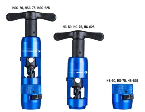
The Jonard all-in-one coring tools provide a complete coring solution for 1/2", 5/8" and 3/4" hardline cables. These tools include a jacket stripper at the front of the tool, a coring tool with an adjustable center conductor beveller and a stop to insure consistent coring lengths with a comfortable ratcheting handle.
