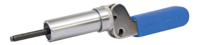
This barrel lock plunger key is the perfect tool for use on Highfield, Channell, and Innertite barrel locks with inside diameters of 0.176" to 0.196". This tool is also compatible with the Channell LK03029817, Highfield 93180775-S, and used in CATV Pedestal Applications. This barrel lock plunger features the following:
