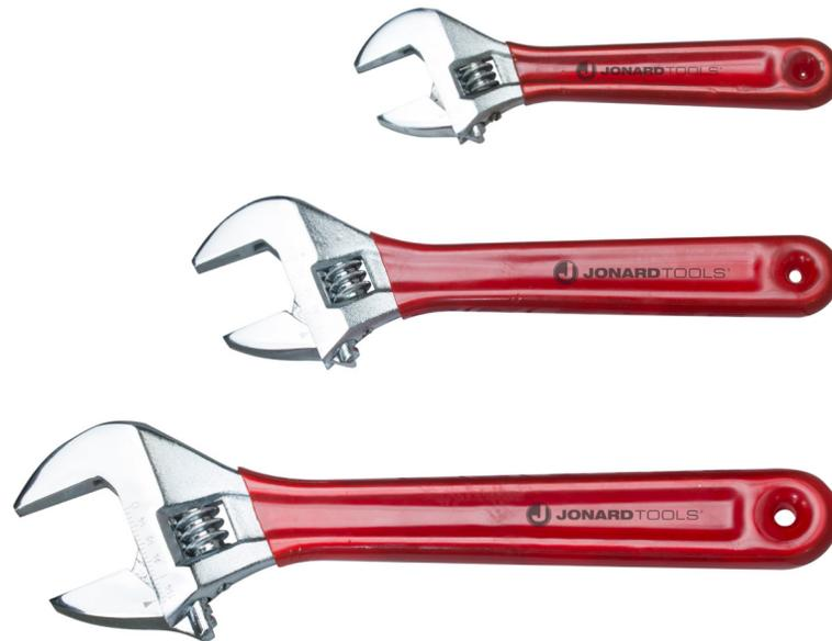
Jonard's adjustable wrenches are made of chrome vanadium steel with a chrome plated finish. They are forged and heat treated for maximum strength. Handles are covered with a red vinyl grip for user comfort. The knurled worm gear is precision formed and the operation is smooth and trouble free. For accurate and faster adjustments use the metric or English scales on either side of the jaws. With extra wide jaws, a smaller wrench works on bigger jobs. Great for tight spaces.
