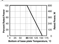
Derating (thermal resistance): 8.33 W/K (0.12 K/W) (for conf. 1, 2, 3) Best results can be obtained by using a thermal transfer compound with a heat conductivity of at least 2.9 W/mK. The flatness of the cooling plate must be better than 0.05 mm overall. Surface roughness should not exceed 6.4  $\mu$ m.
