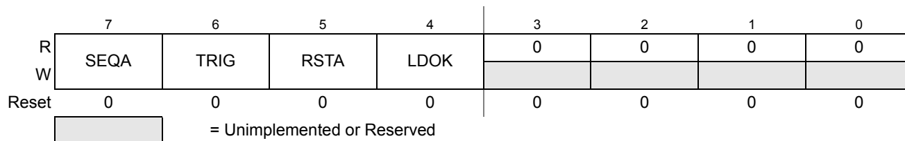
Figure 9-9. ADC Conversion Flow Control Register (ADCFLWCTL)
