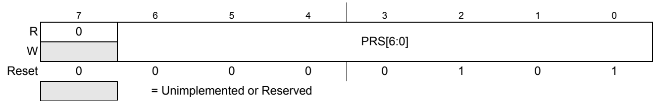
Figure 9-7. ADC Timing Register (ADCTIM))
