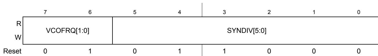
Figure 8-9. S12CPMU_UHV_V10_V6 Synthesizer Register (CPMUSYNR)
