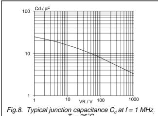
Fig.8. Typical junction capacitance  $C_d$  at f = 1 MHz,  $T_j = 25^{\circ}C$
