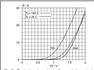
Fig.5. Typical and maximum forward characteristic;  $I_F = f(V_F)$ ; parameter  $T_i$
