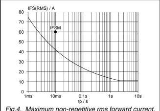
Fig.4. Maximum non-repetitive rms forward current.  $I_F = f(t_p)$ ; sinusoidal current waveform;  $T_j = 150^{\circ} C$  prior to surge with reapplied  $V_{RWM}$ .
