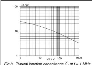
Fig.8. Typical junction capacitance  $C_d$  at f = 1 MHz,  $T_j = 25^{\circ}C$
