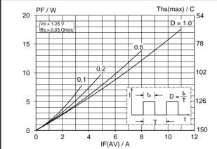
Fig.2. Maximum forward dissipation,  $P_F = f(I_{F(AV)})$ ; square wave current waveform; parameter D = duty  $cycle = t_p/T$ .
