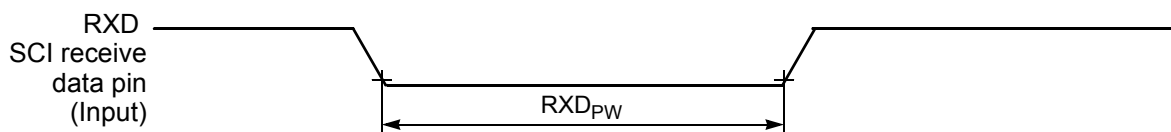
Figure 10-16 RXD Pulse Width
