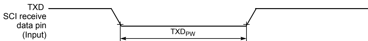
Figure 10-17 TXD Pulse Width
