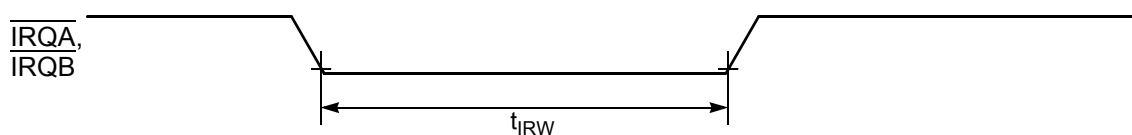
Figure 10-6 External Interrupt Timing (Negative Edge-Sensitive)
