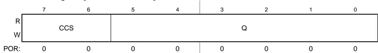
Figure 18-7. RTC Compensation Configure Register (RTCCCR)
