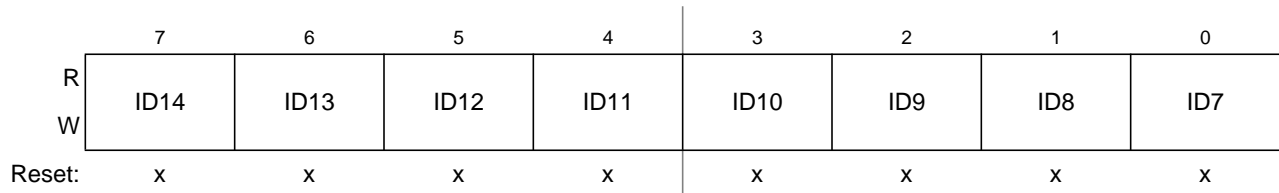
Figure 11-28. Identifier Register 2 (IDR2) — Extended Identifier Mapping
