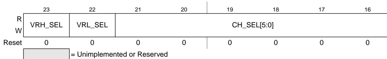
Figure 10-19. ADC Command Register 1 (ADCCMD_1)
