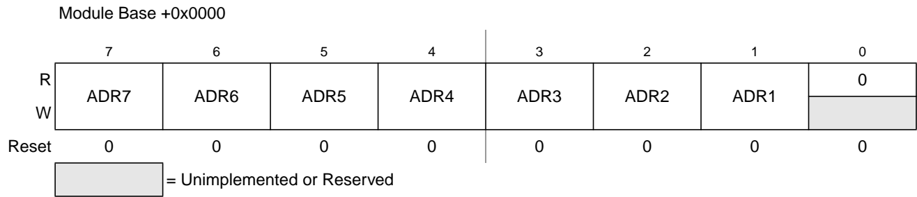
Figure 14-3. IIC Bus Address Register (IBAD)
