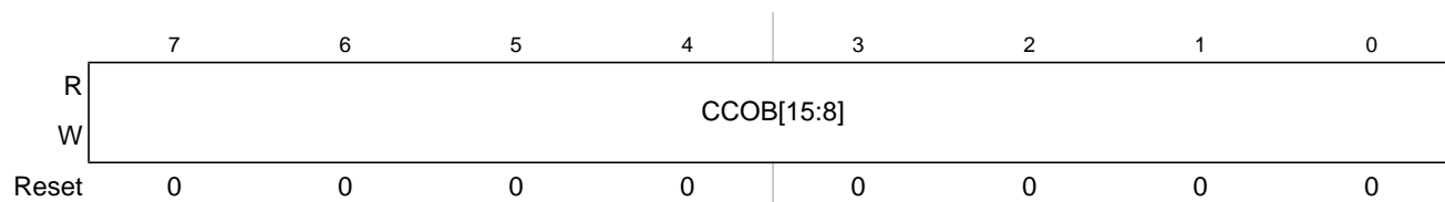
Figure 21-22. Flash Common Command Object 2 High Register (FCCOB2HI)
