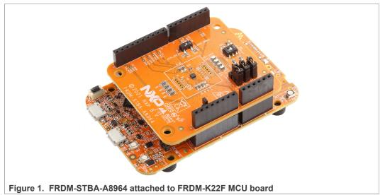
The FRDM-STBA-A8964 shield board kitted with FRDM-K22F helps accelerate sensor evaluation by using the FreeMASTER-Sensor-Tool software tools. This combination of hardware and software enables end users to move through each phase of product
