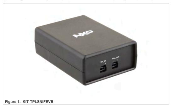
Placed in any TPL bus, it non-intrusively listens to all TPL messages and monitors the frame traffic on the bus (the TPL sniffer works in listen mode only). The corresponding received data (in SPI format) is available on a data output port, to be connected to a logic analyzer and its software which provides further analysis of such data.
