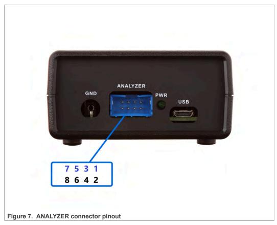
The supplied 8-pin connection cable should be plugged into the ANALYZER connector with the blue wires on top (NXP logo side) and the black wires on the bottom.
