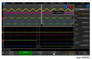
CH1: AC mains (300 V/div) CH2: GATELR (5 V/div) CH3: GATELL (10 V/div) CH4: COMP (5 V/div) Time: 20 ms/div and 10 µs/div
