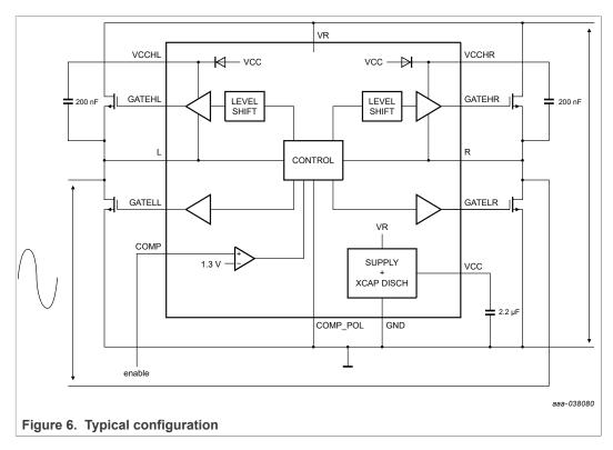
The control circuit of the TEA2209T senses the polarity of the mains voltage between pins L and R. Depending on the polarity, either GATELL or GATELR is switched on. The comparator in the control circuit, which compares the L and R voltages, has thresholds of 250 mV and −250 mV depending on the slope polarity. If the difference voltage between L and R is less than 250 mV both GATELL and GATELR are low.
