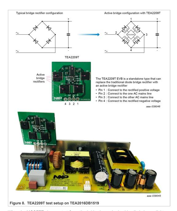
When the MOSFET pin open test for active bridge is required, add a diode in parallel to each active bridge MOSFET.
