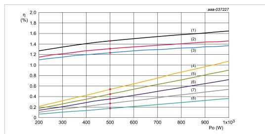
Efficiency drop comparison calculation based on 115 V (AC) input and a die temperature of 125 °C (bridge diode bridge: GSIB15A60;15 A; 600 V; 20 A 600 V).
