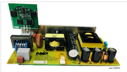
Figure 5. TEA2209DB1584 demo board added to 240 W resonant adapter board
