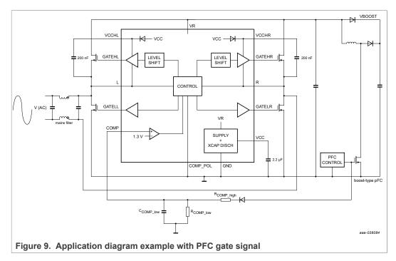
The TEA2209DB1584 implements an external RC filter with  $R_{COMP\_high} = 18 \ k\Omega$ ,  $R_{COMP\_low} = 180 \ k\Omega$ ,  $C_{COMP\_high} = 2.2 \ \mu F$  and 1N4148. To adjust the output power level which disables gate drivers, change  $R_{COMP\_high}$ . As reducing  $R_{COMP\_high}$  value, gate drivers can be disabled at lower power levels. Section 6.8.2 gives the test result with the TEA2016DB1519.
