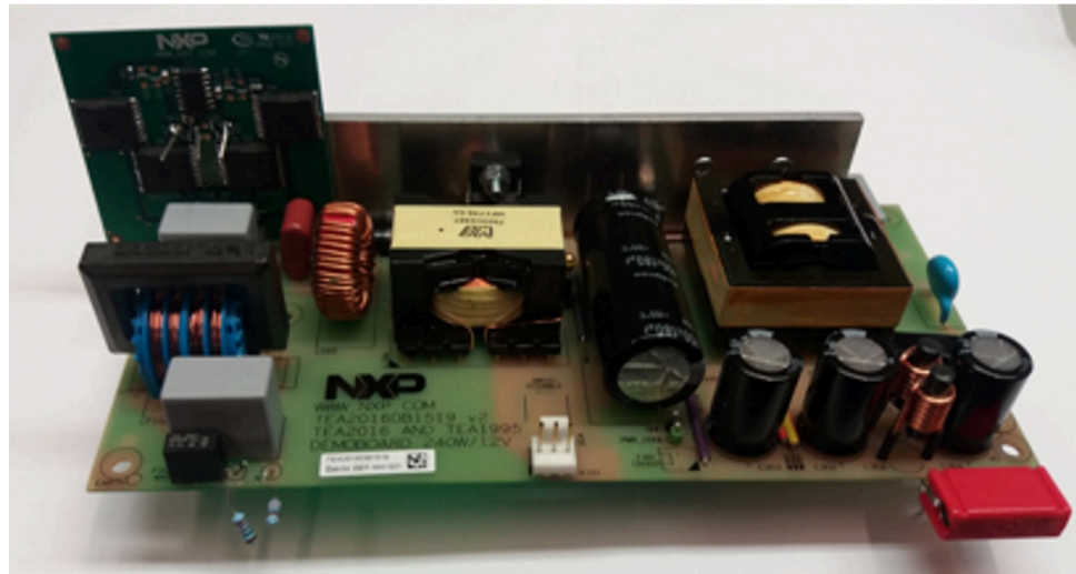
Figure 5. TEA2208DB1576 demo board added to 240 W resonant adapter board
