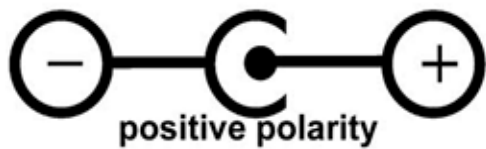
Figure 2-1. Power Supply Barrel Connector (J2) Polarity
