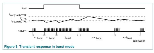
Even though the burst-mode regulates towards a target repetition frequency, the actual repetition rate is lower than the target because of the discrete number of switching cycles. Increasing or decreasing the number of pulses results in a step change in the burst repetition frequency.
