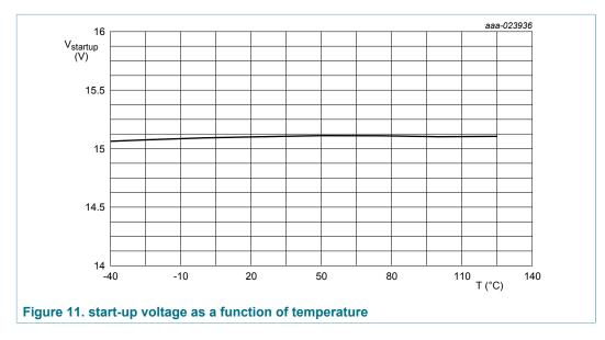
GreenChip SMPS primary side control IC with fixed frequency operation
