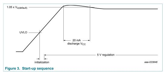
The TEA19032CT operates on supply voltages up to 21 V. The voltage on the VCC pin is used to detect an OVP and UVP. The OVP and UVP level are set as a percentage of the requested output voltage level.
