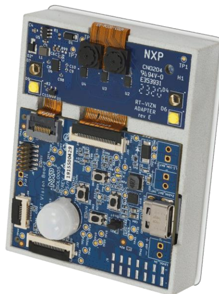
Figure 2: Dual Camera Adapter Kit Configuration
