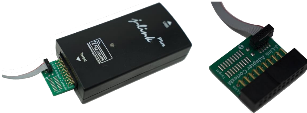
Figure 27: J-Link Plus and 9-Pin Cortex-M Adapter
