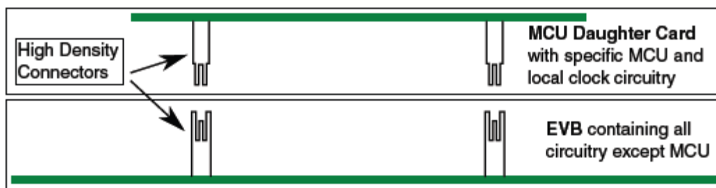
Figure 1. Modular concept – Mother board and MCU daughter card
