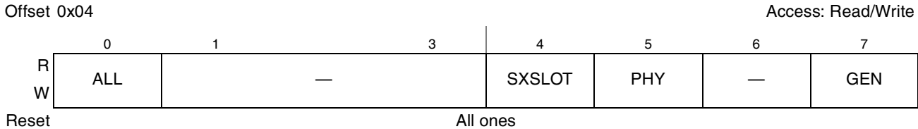
Figure 30. Reset Control Register (PX_RST)
