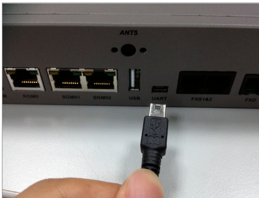
Figure 5. Attaching to a UART Port
