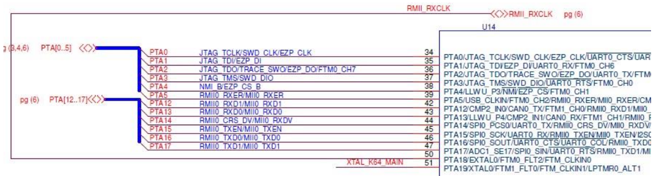
Figure 7. MCU receives RMI clock from Micrel Ethernet PHY
