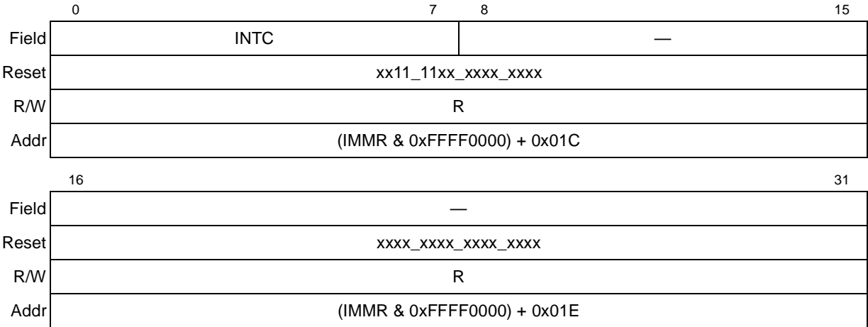
Figure 10-13. SIU Interrupt Vector Register (SIVEC)
