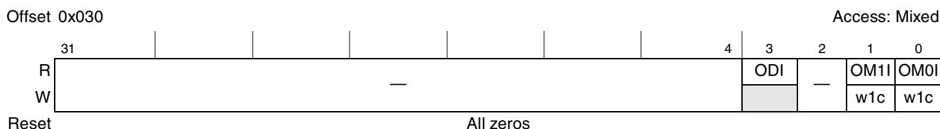
Figure 13-2. Outbound Message Interrupt Status Register (OMISR)
