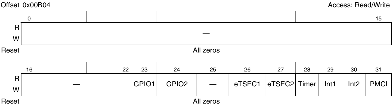
Figure 5-58. Power Management Controller Event Register
