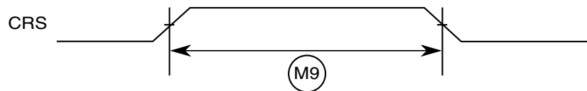
Figure 38. MII async inputs timing diagram
