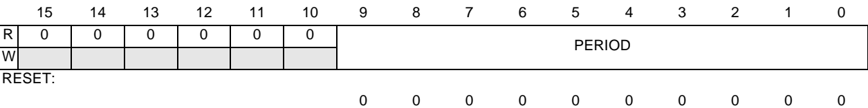
Figure 15-5 PWM Period Registers
