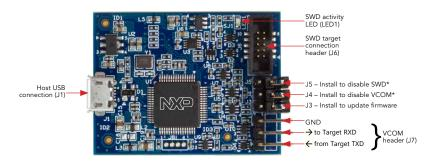
\*J4 and J5 jumper headers may not be installed on all boards.
