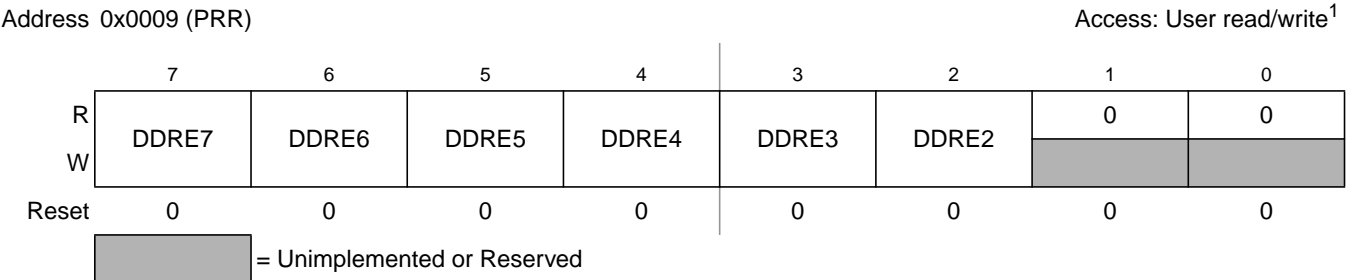
Figure 2-7. Port E Data Direction Register (DDRE)
