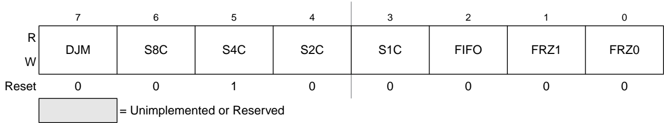
Figure 10-7. ATD Control Register 3 (ATDCTL3)
