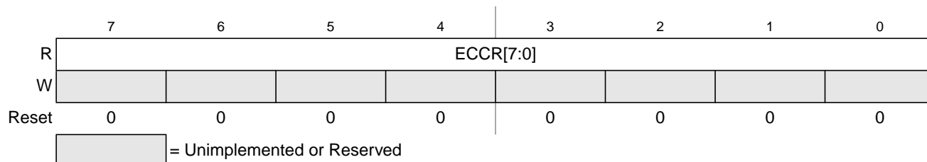
Figure 20-21. Flash ECC Error Results Low Register (FECCRLO)
